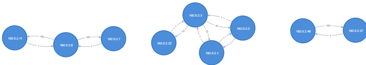
Figure 5: MATCH (u:ROUTER)-[e1:LINKED]->(v:ROUTER) MATCH (v)-[e2:LINKED]->(u) WHERE e1.cost <> e2.cost AND id(u)<id(v) RETURN u, v
